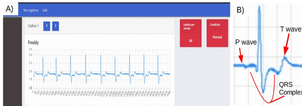
Figure 4: A) Screen shot of the user interface B) Ampliation of a single ECG cycle with waves and complex labeled
