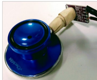
Figure 3. Electret microphone module attached to the commercial stethoscope bell
