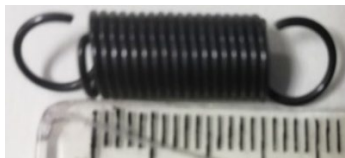
Figura 1: Resorte SMA 0.75 mm
